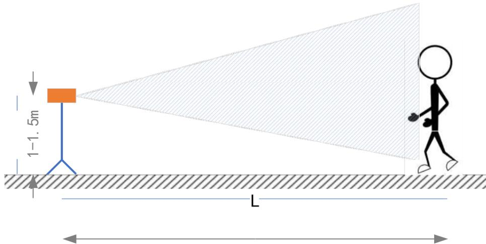
Figure 2 Horizontal installation
