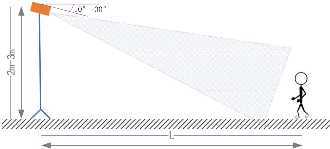
Figure 3 Inclined installation
