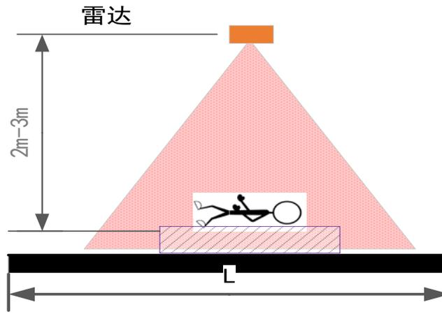
Figure 4-2 Top installation detection
