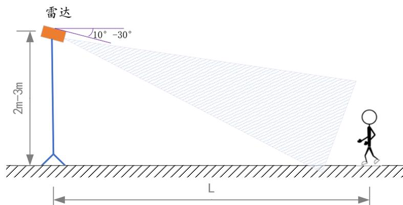
Figure 4-2 Detecting diagram of oblique installation
