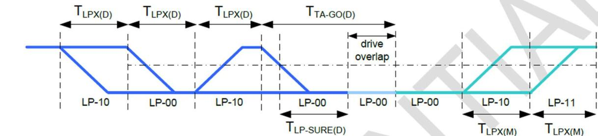
Bus turnaround (BAT) from display module to MPU timing
