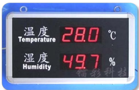
Temperature and Humidity Board
