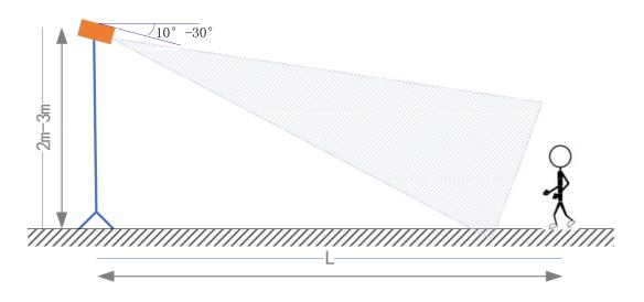
Figure 3 Inclined installation
