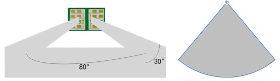
Figure 1 Schematic diagram of radar coverage area
