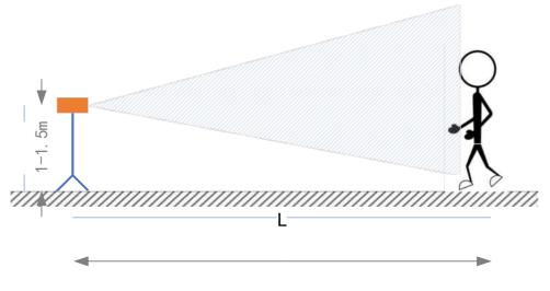
Figure 2 Horizontal installation
