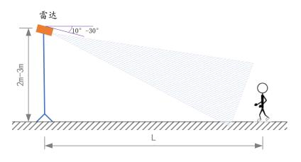
Figure 4-2 Detecting diagram of oblique installation
