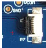
Figure 5 : Connection between DESPI-C03 and front light panel
