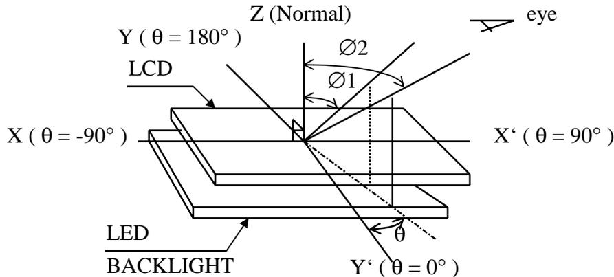
NOTE (2) : DEFINITION OF VIEWING ANGLE  $\Phi 1$  AND  $\Phi 2$
