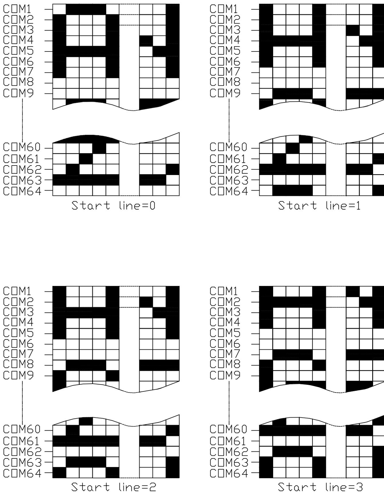
Fig.7 Relation Between Start Line and Display
