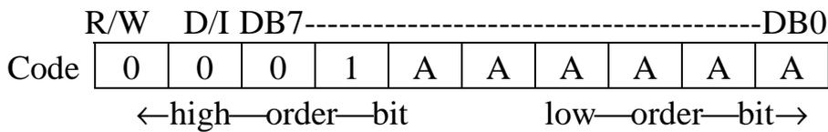
Y address AAAAAA (binary) of the display data RAM is set at the Y address counter. After that, Y address counter is increased by 1 every time the data is written or read to or from MPU.
