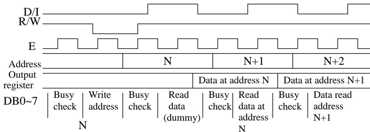
Fig.5 CPU Read Timing
