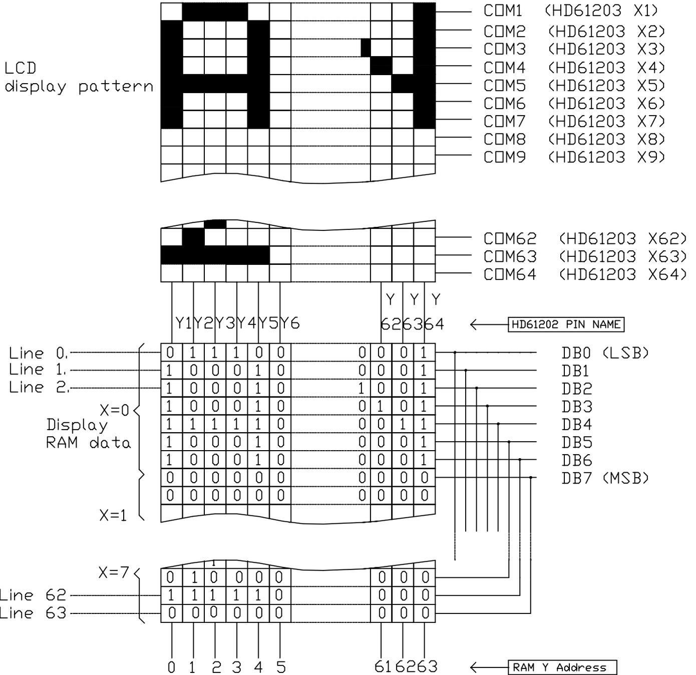
(a) ADC="1" (Connected to Vcc)
