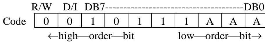
X address AAA (binary) of the display data RAM is set at the X address register. After that, writing or reading to or from MPU is executed in this specified page until the next page is set.
