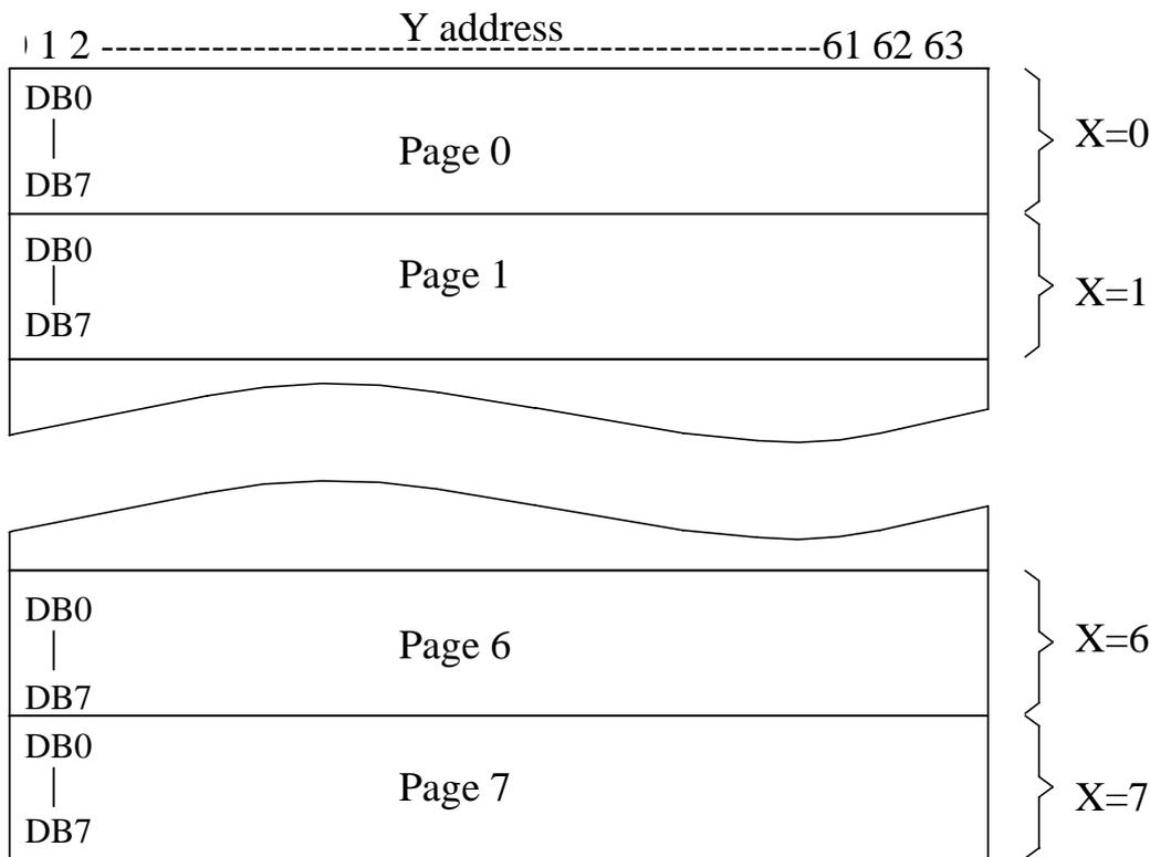
Fig. 8 Address Configuration of Display Data RAM
