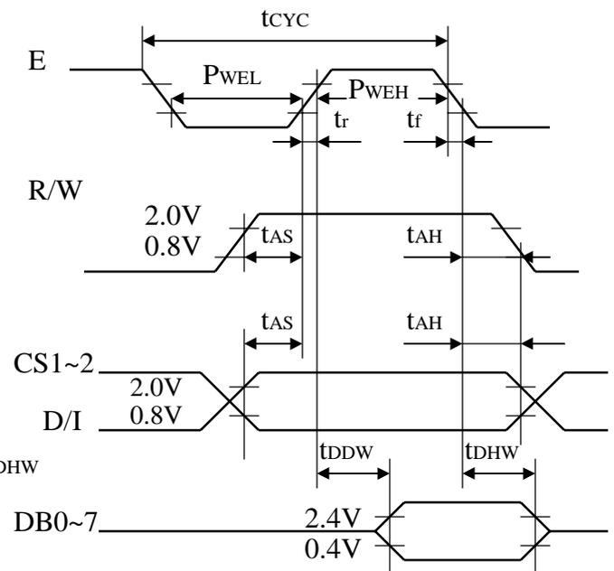
Fig . 2 CPU Read Timing
