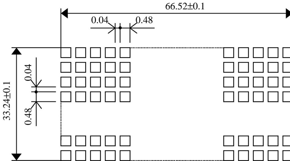
NOT SPECIFIED TOLERANCE: ±0.01mm
