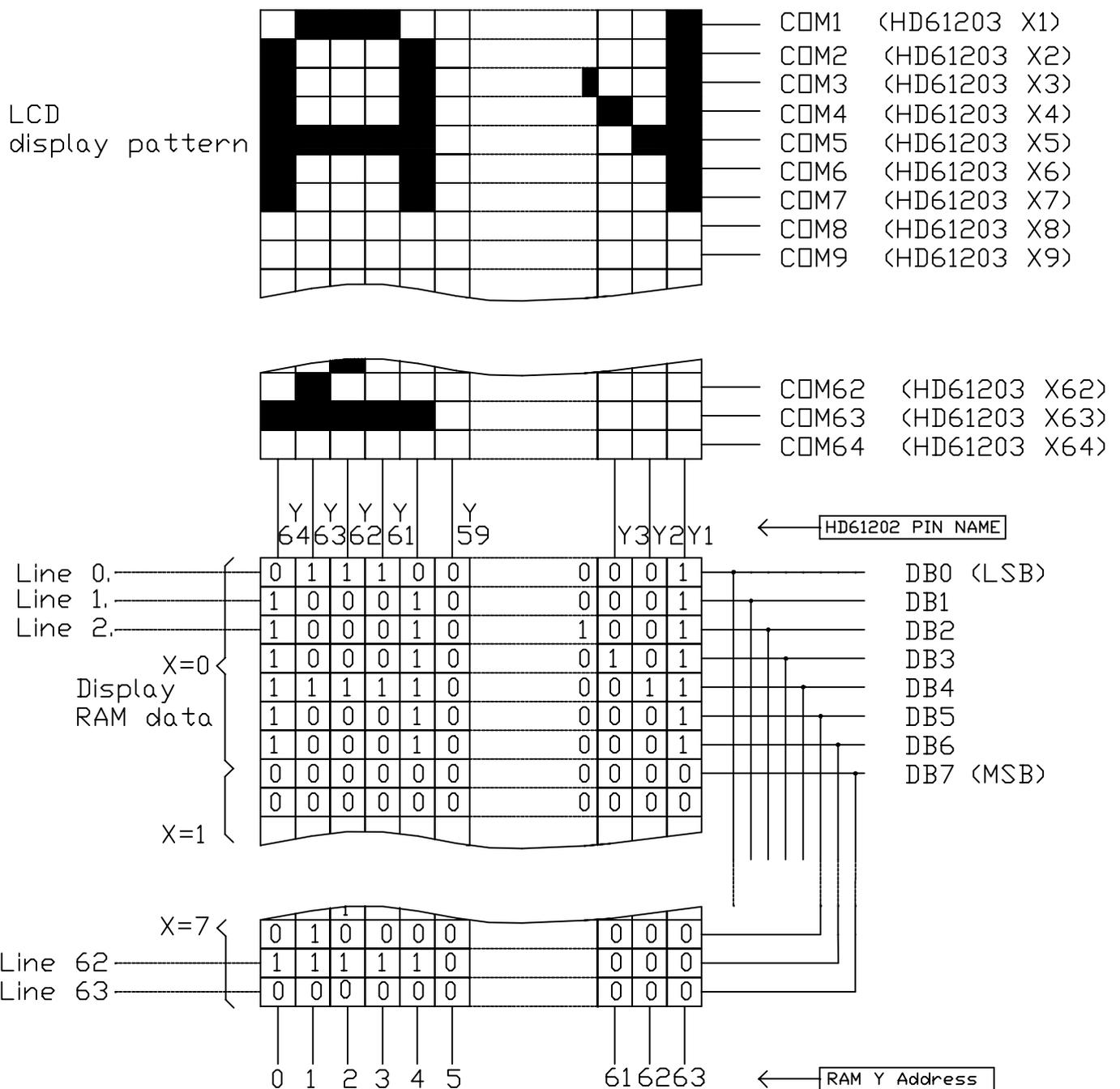
(a) ADC="0" (Connected to GND)
