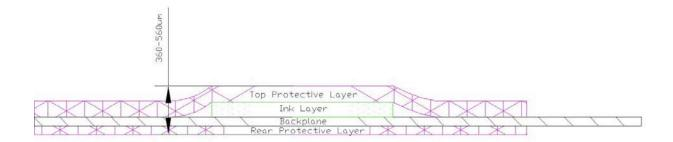
Each segment on an E Ink display has an individual electrode on the back plane. Each electrode is routed on the back plane, forming a display connector or tail off the edge of the display. For a Segmented Display Cell (SDC), the tail includes one trace for each segment plus two additional traces for top plane and back plane connection. For example, if your display uses 96 segments, the tail would include 98 traces or pin outs.
