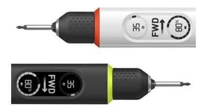
Example of an E Ink Segmented display (left) compared to a traditional segmented LCD:
